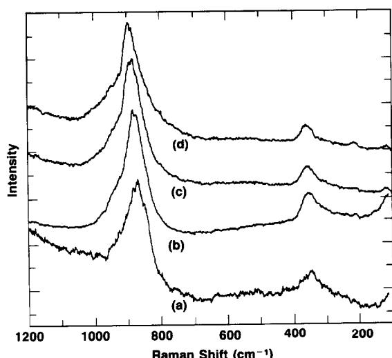
Fig. 3. Raman spectra of chromium oxide supported on alumina, calcined at 500 °C, as a function of chromium oxide coverage; (a) 0.5%  $\text{CrO}_3$ , (b) 1%  $\text{CrO}_3$ , (c) 3%  $\text{CrO}_3$ , (d) 5%  $\text{CrO}_3$ .
