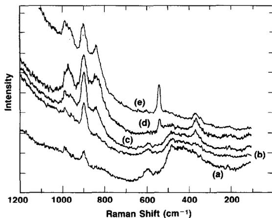
Fig. 9. Raman spectra of chromium oxide supported on silica, calcined at 500 °C, as a function of chromium oxide coverage; (a) 0.2%, (b) 0.5%, (c) 1%, (d) 3%, (e) 4% CrO<sub>3</sub>.
