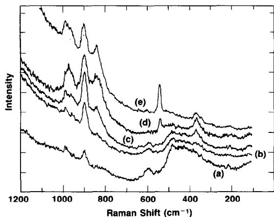
Fig. 9. Raman spectra of chromium oxide supported on silica, calcined at 500 °C, as a function of chromium oxide coverage; (a) 0.2%, (b) 0.5%, (c) 1%, (d) 3%, (e) 4% CrO<sub>3</sub>.
