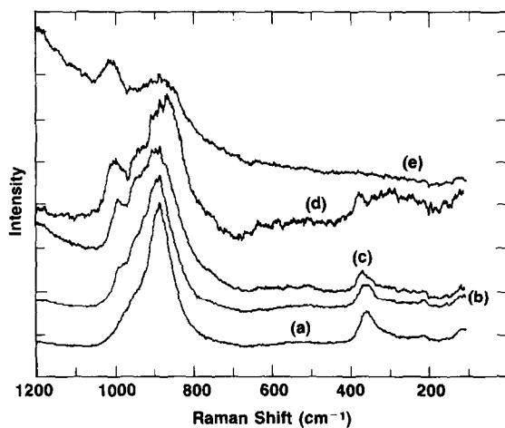
Fig. 5. Raman spectra of laser-induced dehydration of 3% CrO<sub>3</sub>/Al<sub>2</sub>O<sub>3</sub>: increasing laser power from (a) to (e).
