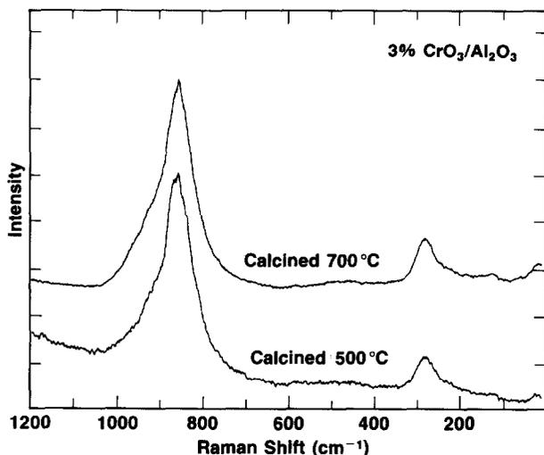
Fig. 4. Raman spectra of 3% CrO<sub>3</sub>/Al<sub>2</sub>O<sub>3</sub> as a function of calcination temperature.
