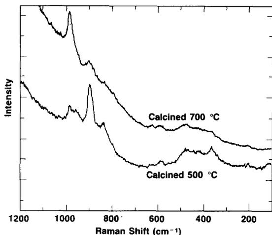
Fig. 10. Raman spectra of 1%  $\text{CrO}_3/\text{SiO}_2$  as a function of calcination temperature.
