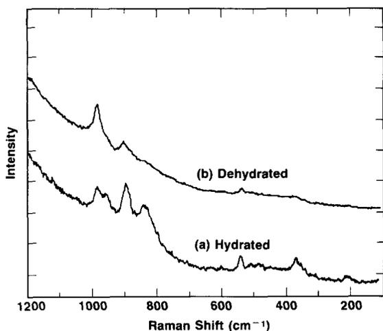
Fig. 11. Raman spectra of laser-induced dehydration of 3%  $\text{CrO}_3/\text{SiO}_2$  calcined at 500 °C.
