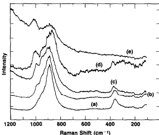
Fig. 5. Raman spectra of laser-induced dehydration of 3%  $\text{CrO}_3/\text{Al}_2\text{O}_3$ : increasing laser power from (a) to (e).
