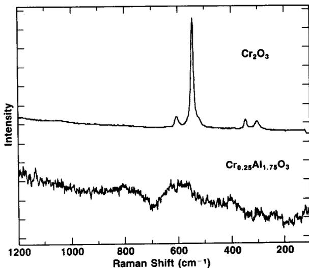
Fig. 2. Raman spectra of solid chromium(III) oxides.
