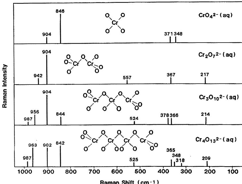
Fig. 1. Raman spectra of aqueous chromium(VI) oxides.
