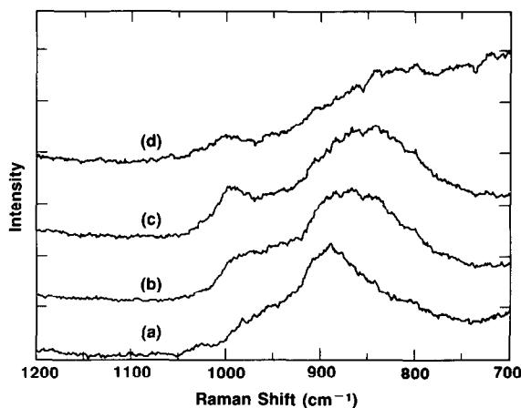
Fig. 8. Raman spectra of laser-induced dehydration of 4%  $\text{CrO}_3/\text{TiO}_2$  calcined at 500 °C; increasing laser power from (a) to (d).
