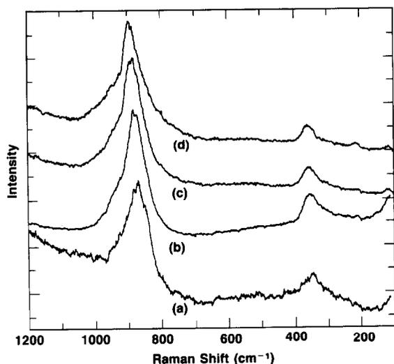
Fig. 3. Raman spectra of chromium oxide supported on alumina, calcined at 500 °C, as a function of chromium oxide coverage; (a) 0.5% CrO<sub>3</sub>, (b) 1% CrO<sub>3</sub>, (c) 3% CrO<sub>3</sub>, (d) 5% CrO<sub>3</sub>.
