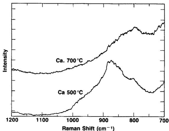
Fig. 7. Raman spectra of 1% CrO<sub>3</sub>/TiO<sub>2</sub> as a function of calcination temperature.
