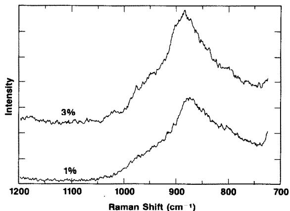
Fig. 6. Raman spectra of chromium oxide supported on titania, calcined at 500 °C, as a function of chromium oxide coverage.
